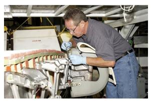
United Space Alliance worker Mike Hyatt attaches a Reinforced Carbon-Carbon (RCC) panel onto the leading edge of the wing of the orbiter Atlantis.
